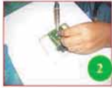
Relay assembly and soldering using jig
