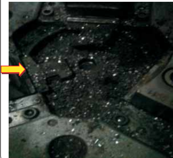
Scrap and sand inside the chuck
